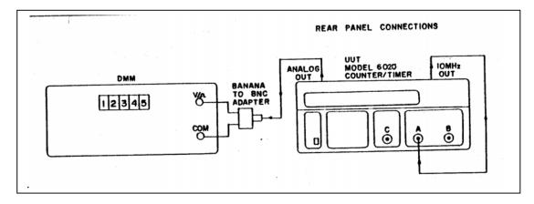
Figure 5-15. Analog Output Test Set-up.
