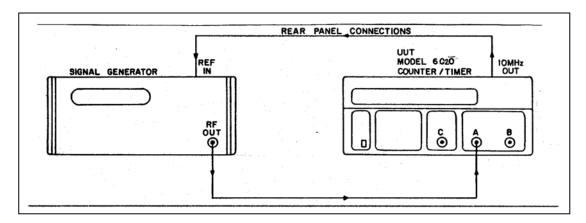
Figure 5-7. Period A and Period A Averaged Test Set-up.
