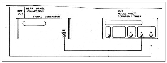
Figure 5-8. Ratio A/B Test Set-up.
