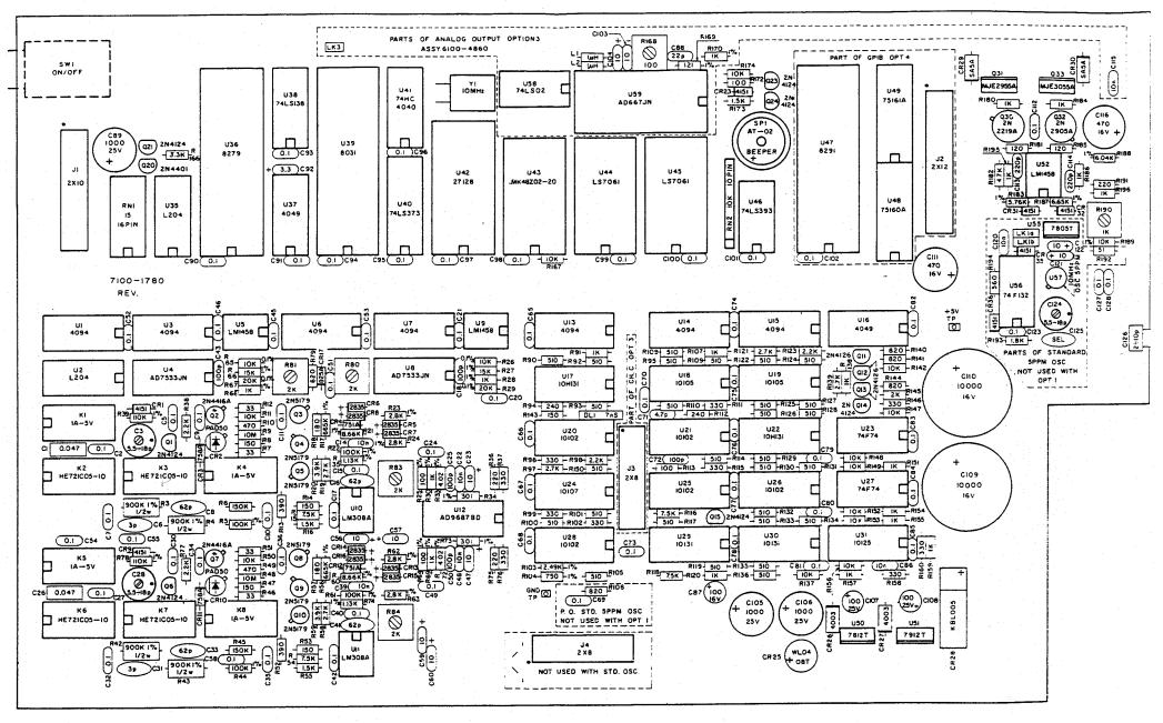
Figure 9-6. Main Board - Components Location Diagram
