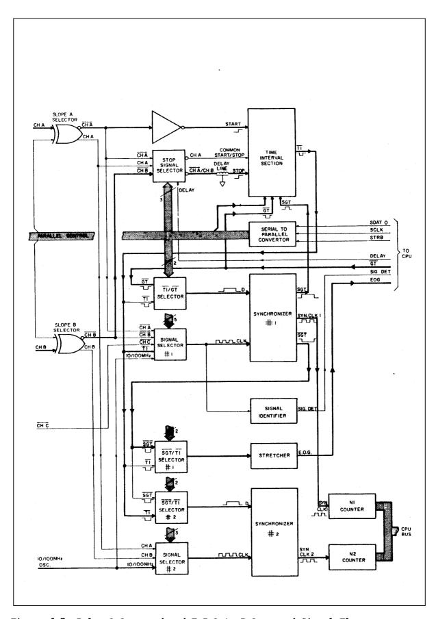
Figure 6-7. Pulse A Averaged and T.I A to B Averaged Signal Flow Diagram.
