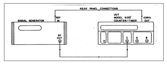
Figure 5-6. Channel C Sensitivity Test Set-up.
