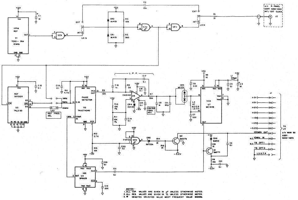
Figure 9-9. Option 1 - TCXO and x10 Multiplier Circuit
