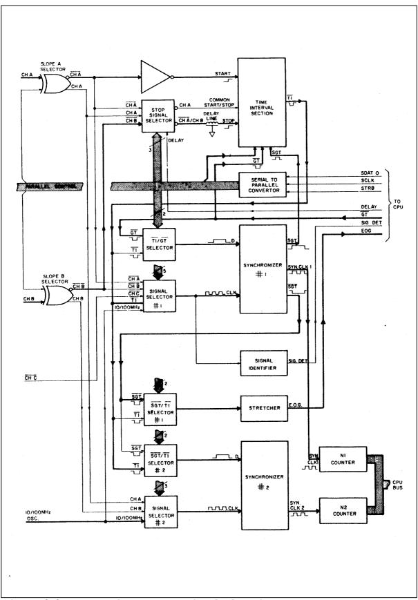
Figure 6-6. PER A and T.I A to B Signal Flow Diagram.
