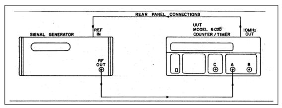
Figure 5-5. Channels A and B Sensitivity Test Set-up.
