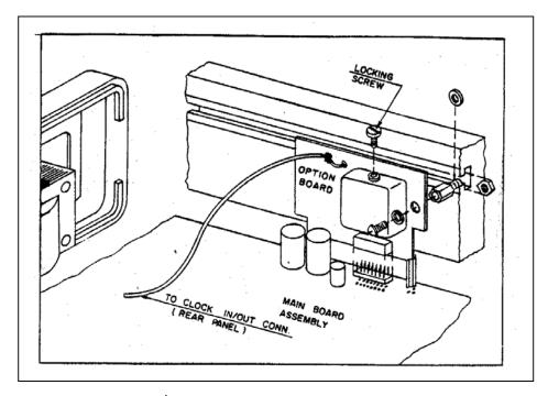
Figure 5-1. TCXO/Clock Multiplier Option Field Installation.
