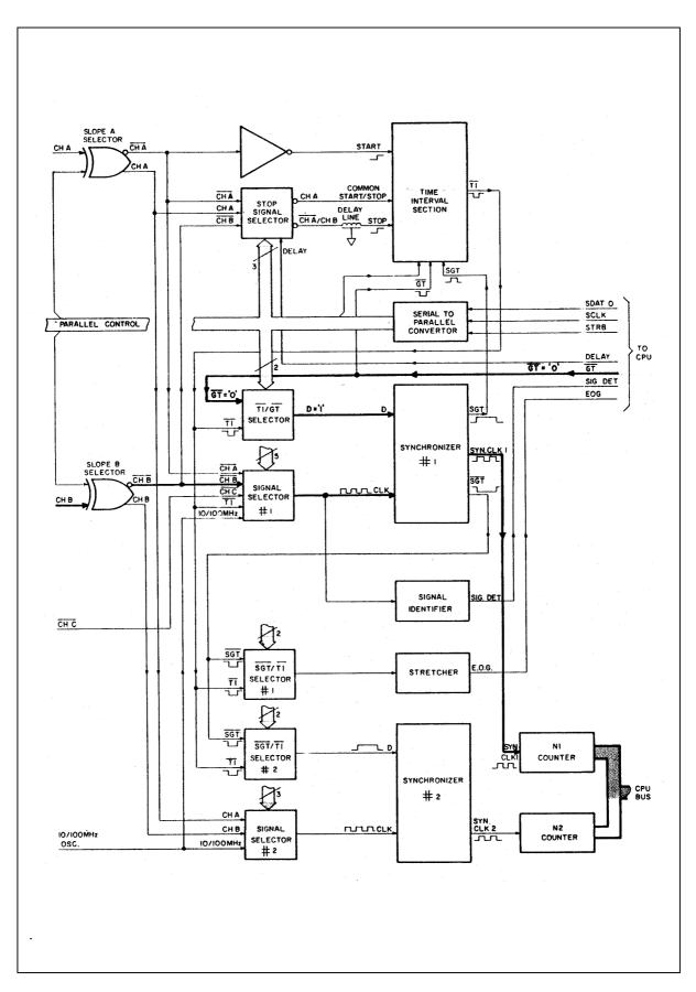
Figure 6-8. Totalize B Infinite Signal Flow Diagram.
