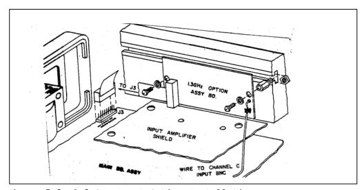
Figure 5-3. 1.3 GHz Input Option Installation
