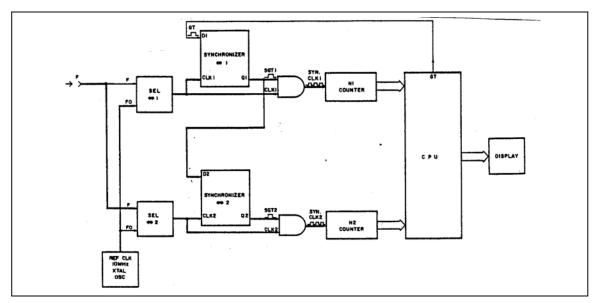
Figure 6-2. Conventional Frequency Measurement.
