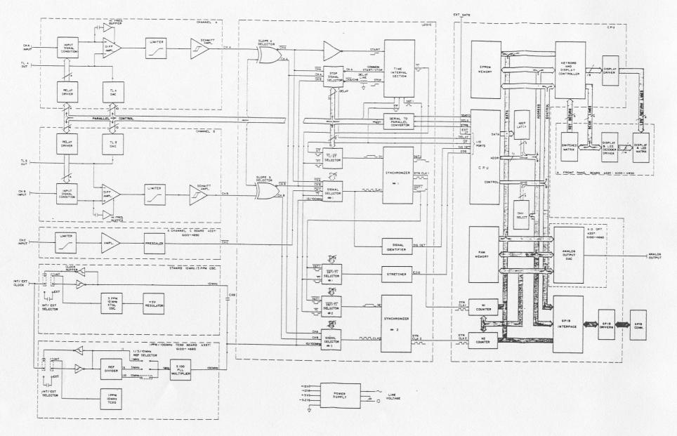
Figure 5-3. Model 6020 - General Block Diagram
