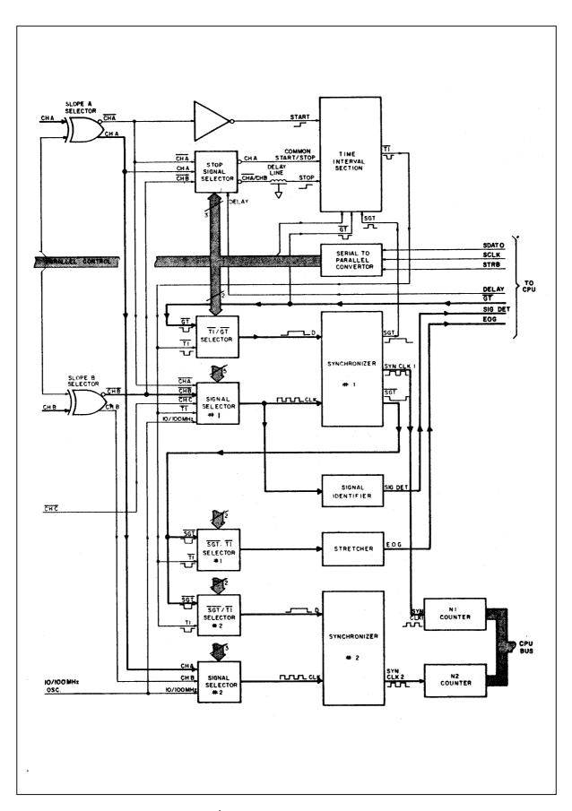
Figure 6-5. Frequency Ratio A/B Signal Flow Diagram.
