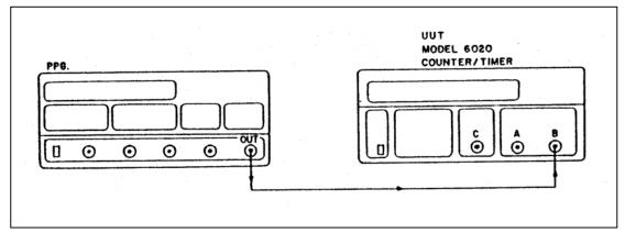
Figure 5-11. Totalize B Test Set-up.
