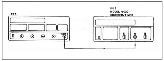
Figure 5-12. Auto Trigger A and B Test Set-up.
