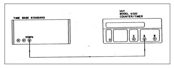
Figure 5-16. Time Base Accuracy Test Set-up.
