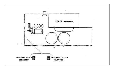
Figure 5-4. External/Internal time base clock selection
