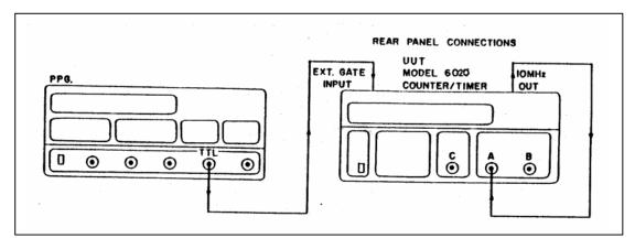
Figure 5-14. User Gate Test Set-up.
