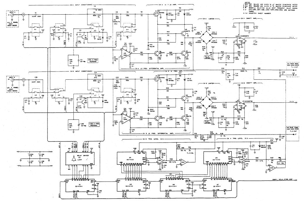
Figure 9-1. Main Board - Input Amplifiers and Trigger Level Control
