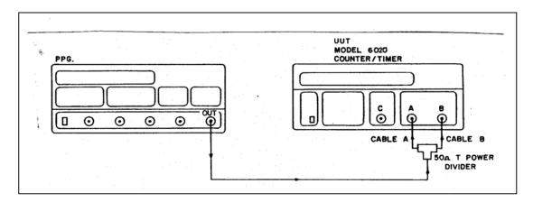
Figure 5-9. Pulse A, T.I A to B and Averaged Test Set-up.
