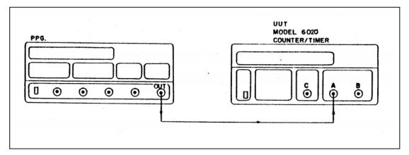
Figure 5-13. Delay Test Set-up.
