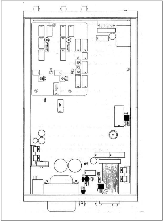
Figure 7-1. Model 6020 Adjustment Points Location.
